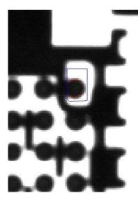
**Dispense Tool:** This tool measures the total dispense size for the pad, and for the individual lead. This includes all dots. Any variation in the viscosity of the past, temperature etc. is recognized. This tool monitors the "global" dispense process, and generates an alarm if these parameters are out of spec.
