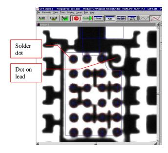
The dots may have some flux material around. The system ignores the flux, and calculates each dot size, its densitometric volume, its position (centering to the pad)with reference to its "ideal" position (defined in the CAD cluster table).
