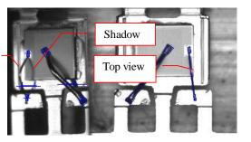
This special combination of shadow / wire allows to execute loop height inspection. Result is detection of
