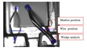
See the difference between good bond (left) and partially lifted one (right):
