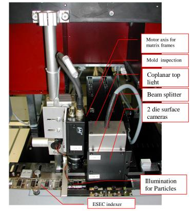
Integration into an existing ESEC wire bonder (camera replaces bond head) allows an easy and reliable handling for any standard leadframe type. The handling also is compatible to the ESEC AutoLine. And the user can re-utilize any type of ESEC wire bonder (also old models) to re-use for this purpose of quality control.
