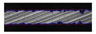
The system finds the true die edge contour including all chipping effects. The average wafer thickness is calculated. Chipping is localized on the edge automatically. Chipping is separated into shell and deep cracks. While flat shell chips are uncritical, the hard cracks go deep into the material, and are a possible starting point for micro cracks of the material.
